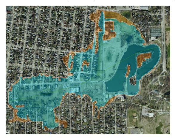
The proposed mitigation action would be to construct a storm sewer to provide positive drainage from the depressional area. The project is expected to protect thirty-eight low-to-moderate income homes and four roads from flood damage. Preliminary engineering has been completed, and the project is expected to cost \$1,100,000 and could be completed in 12-18 months. The cost could be covered by a combination of local contribution, Aurora Township, Kane County, and FEMA.
