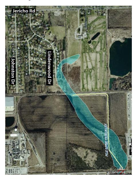
A flood study of the area and concept level engineering has been completed for a project to resculpt the topography on an adjacent 5-acre farm parcel to the east of Lindenwood Drive and create a detention storage for floodwaters that previously impacted the neighborhood. The project is expected to alleviate flooding for nine or more homes and two roads. The project is
