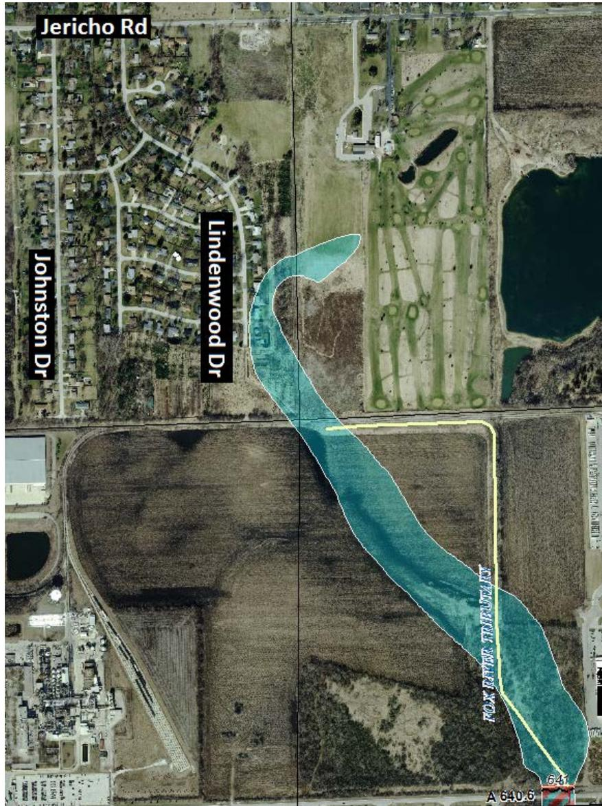
A flood study of the area and concept level engineering has been completed for a project to resculpt the topography on an adjacent 5-acre farm parcel to the east of Lindenwood Drive and create a detention storage for floodwaters that previously impacted the neighborhood. The project is expected to alleviate flooding for nine or more homes and two roads. The project is
